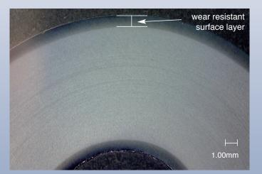
Round steel chains operating in slaughterhouse lines are exposed to chemical influences, such as cleaning agents, and therefore under constant corrosion attack. Alloy, steel chains of this kind are provided with a galvanic coating to counteract the effect of corrosion. The professionally applied, galvanic surface sealing that THIELE has been employing for many years effectively counteracts premature corrosion.
